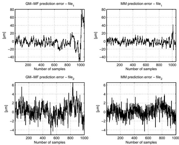
Fig. 6. Prediction errors  $h_2(\kappa) - \hat{h}(\kappa)$ : left plots for GM-MF prediction, right plots for MM prediction, for file<sub>1</sub> and file<sub>2</sub> respectively.
