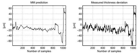
Fig. 5. MM prediction and the measured thickness deviation for file<sub>1</sub>. The measured value was shifted appropriately to allow direct comparison.
