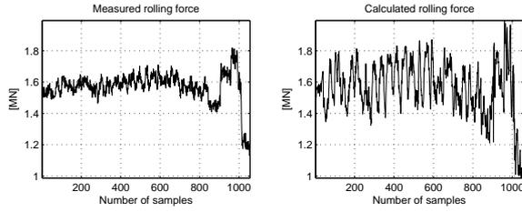
Fig. 2. Comparison of the rolling force  $F$  measured directly by the force sensor and  $F_p$  calculated from hydraulic pressures.
