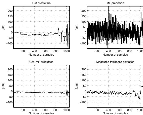
Fig. 3. Predictions made according to classical relations GM and MF compared with the GM-MF prediction and the measured thickness deviation for file<sub>1</sub>. The measured value was shifted appropriately to allow direct comparison.
